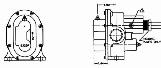
CREASE FITTINGS (ITEM 17) INSTALLED INTO .125-27 NPT CONNECTIONS.
